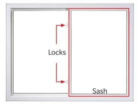
The steps below will guide you through removing your current slider window sash and installing your new window sash. The diagram to the left illustrates the parts of the window to help you complete your window sash replacement.
